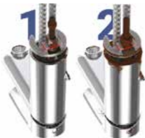
PICTURE 1: Results of the cathodic protection patented by Ramon Soler® after 600 hours salt spray.
