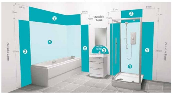
**Zone 1** refers to the area above the shower up to a height of 2.25 metres and requires a minimum rating of IP44 or higher and if the fitting is 240V a 30ma RCD must be used to protect the circuit.
