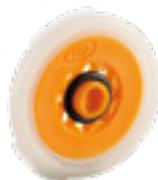
Economy shower regulator suitable for accurate flow control to mains pressure feed systems only. Can be fitted in any 1/2" flat face connection, shower hose or flexible tap connectors. Come complete with integral gasket. Available in 6.0 litre, 8.0 litre, 10.0 litre or 12.0 litre flow rates
