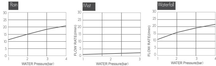
Aquamist ceiling mounted overhead shower, with mist, cascade and rain feature. Separate remote for colour control and chromo therapy, HP 2
